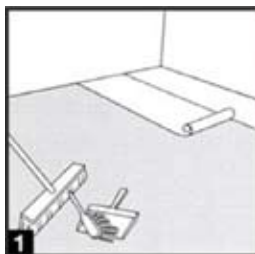
1. After cleaning the sub floor you can roll over the underlay. The underlay has to overlap 20-30cm (7 7/8" - 11 13/16").
