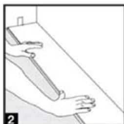
2. Begin laying in the left-hand corner. Place the floorboard 10 mm (3/8") from the left wall. Use spacers between the wall and the floorboard.
