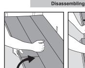
Separate the whole row by carefully lifting up and releasing the whole row. Fold up and release the whole long side.
