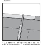
10. Lastrow (and perhapsals of irst row). Minimum width 2" (50mm). Remember expansion gap of 3/8" (10mm).
