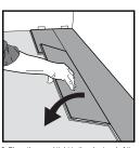
Place the panel tight to the short end of the previous panel and fold down in a single action movement
